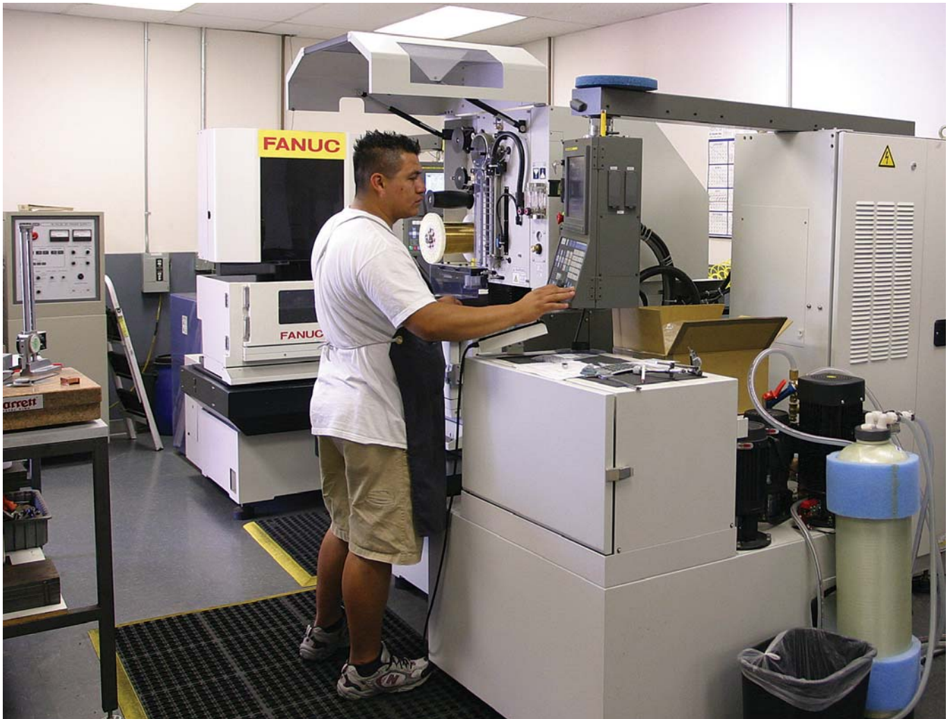
John Colunga, EDM operator, sets up Barrot's newest wire EDM system, a Fanuc XOC. Barrot operates 6 Fanucs and one small Brother EDM machine. The department is run by James Barrot, the middle of the three brothers.
